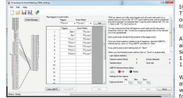
In this simple example up to 7 TTL event marks will be made once paired with an input
