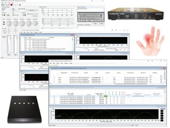
Finished in an attractive carbon fiber effect our response pad houses up to 5 pressure/force sensitive buttons with clear keycaps. If you opt for a custom laser cut solution you are free to design your own button layout to make your response pad truly bespoke to you.
